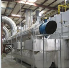
Regenerative Thermal Oxidizers installed at our plants have reduced the amount of energy it takes to cure our products and reduced CO<sub>2</sub> emissions from the curing ovens by up to 90%.
