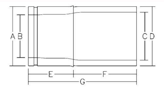
Fully pressure rated • Standard SDR sizes 7,9,11,17 Manufactured to D1599, D1598, D3350 11/00 ® Registered Trademark Poly-Cam, Inc. - US Patent # 5,211,429
