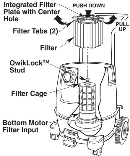
2. Align the small center hole in the top of the filter over the Qwik Lock™ stud on the filter cage. Press firmly on top of the filter near the stud to allow the filter to snap over the ball on the end of the stud. The filter is now attached.
