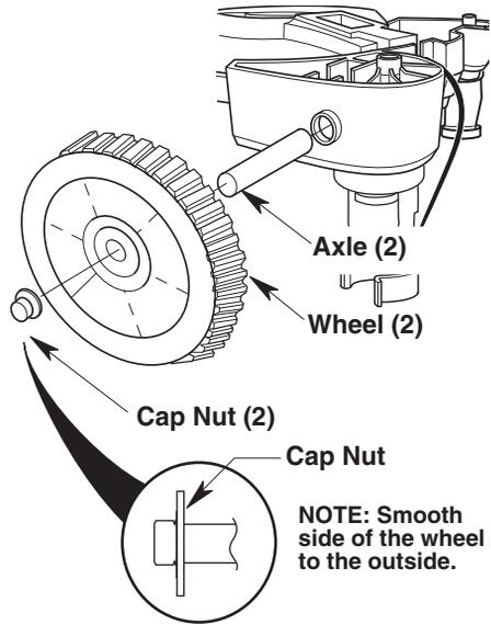
2. Slide the open end of the axle through the hole in the side of the power base until it stops. Install the axle retainer over the axle with the two screws provided.
