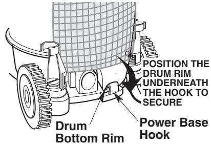
4. Lower the front of the drum onto the power base and slide drum lock lever to locked position to secure.
