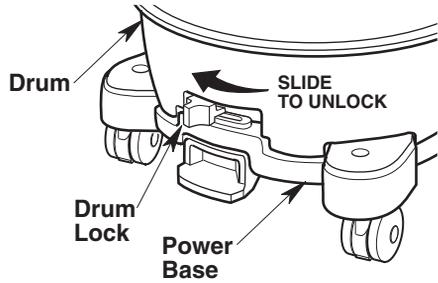
2. Lift up on the drum, using the lift handle found on the lid of the drum. Allowing the front of the drum to come up first will cause the drum to smoothly and properly disengage from the power base.
