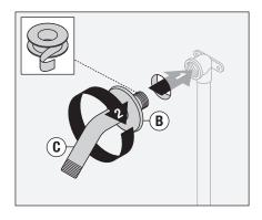
6) Install showerhead (A) to shower arm (C) turning clockwise to tighten.
