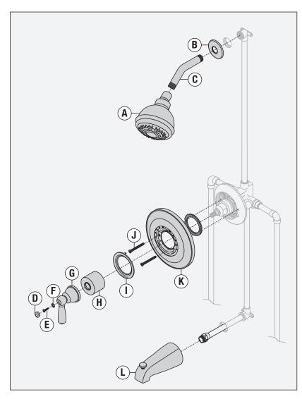
\*Note: Apply a bead of silicone around the perimeter of the escutcheon after installing trim flush with wall. Leave opening on bottom of escutcheon for weep hole.
