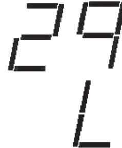
Active Protection – Code 29L – Open high pressure control
