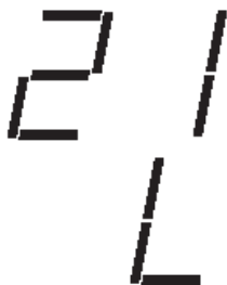
Active Protection – Code 21L – Open low pressure control
