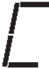
Flashing upper case C A call for second stage cooling has been received
