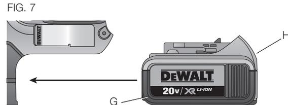
To remove the battery pack from the tool, press the release button (H) and firmly pull the battery pack out of the tool handle. Insert it into the charger as described in the charger section of this manual.
