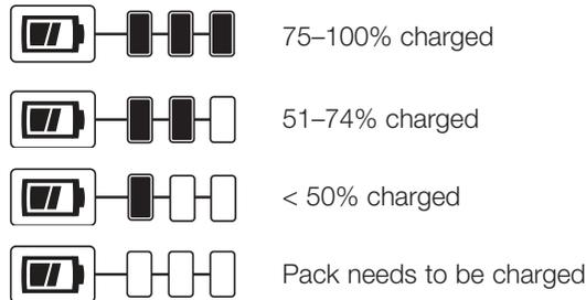
To actuate the fuel gauge, press and hold the fuel gauge button (M). A combination of the three green LED lights will illuminate designating the level of charge left. When the level of charge in the battery is below the usable limit, the fuel gauge will not illuminate and the battery will need to be recharged.
