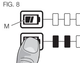
**NOTE:** The fuel gauge is only an indication of the charge left on the battery pack. It does not indicate tool functionality and is subject to variation based on product components, temperature and end-user application.
