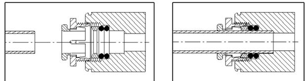
Note: Screw the locknut hand tight to seal
