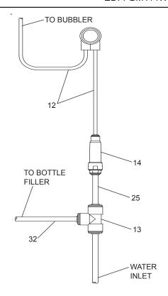
Figure 2 - EZWS-EDFPBM114K Tube Routing
