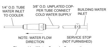
Figure 11 – Water Supply Connections
