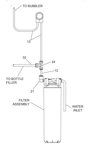
Figure 3 - LZWS-EDFPBM114K Tube Routing
