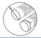
Measure the pipe's outside diameter and make sure the coupling's size fits properly.
