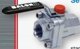
Balon continues as an innovator in valve design with the extension of our Series F threaded end ball valve. The forged body and adapter with rugged bolted construction ensures optimum performance in the field. 316 stainless steel ball and stem. NACE standard. Available in 1/4" through 1"- 3000 PSI. Also offered in LF2 for low-temp service to -50° F.
