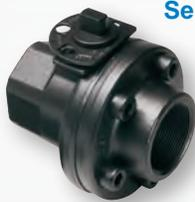
Available in sizes from 1" through 4", with pressures up to 5000 PSI WP. Firesafe design and built in locking device are standard. Bolted body construction protects against end adapter blowout. Offered in carbon steel, nickel aluminum bronze and ductile iron. Also available in LF2 for low-temp service to -50° F.
