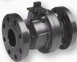
Available in sizes up to 6" and offered in ANSI 125, 150, 300, 600, 900 and 1500 pressure classes. Because it is totally maintenance free, it eliminates the expense of lubrication and grease contamination in meters and other equipment. This valve is available in ductile iron and carbon steel. Also available in LF2 for low-temp service to -50° F.
