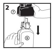
While still pushing the green release latch, pull downward on the refill bottle () and remove it from the motor assembly/bottle support ().
