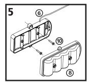
If using a battery box, remove the cover ® by loosening the two captive screws on the battery box cover. position the box on a convenient (vertical or horizontal) surface under the counter top that will allow access for battery changing. Attach the box to the surface using the two screws: ① and anchors: (if attaching to a plaster or masonry surface). Use the wall clip (not shown) to secure the power cable to a wall or other under-counter surface if desired.
