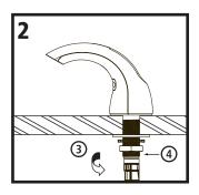
From underneath the counter, first feed the washer ② and then the mounting nut ③ over the data cable ⑤ and onto the threaded stem of the dispenser assembly ①. Tighten the nut securely.
