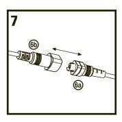
Connect the Power Connector to battery box or AC adaptor.
