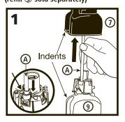
Snap in dispenser straw (A) (see inset). Feed the dispenser straw (A) on the refill bottle (9) up through the motor assembly/bottle support (7) and dispenser assembly (1), aligning the two indents in the bottle and the support. Slide the bottle upward until it snaps into place.
