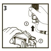
Align the indent inside the top of the motor assembly/bottle support with the indent on the stem of the dispenser assembly and firmly push the motor assembly/ bottle support up, onto the stem.
