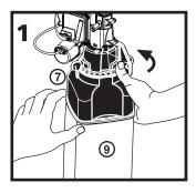
Grasp the empty refill bottle (9) with one hand and use the other hand to push the green release latch on the motor assembly/bottle support (7) to the right (counterclockwise as seen from above).
