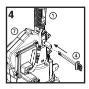
Secure the motor assembly/bottle support to the dispenser assembly stem by pushing the retaining dip into place through the vertical slots, until it goes all the way through the motor assembly.
