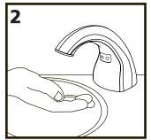
Test the system by passing your hand under the spout of the dispenser assembly ① (in front of the sensor window) three or four
