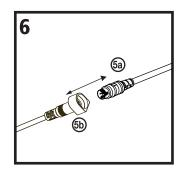
Connect the two halves of the data cable (5a) and (5b) by lining up the white stripes on each half and pushing the cable connectors together until the stripes touch.
