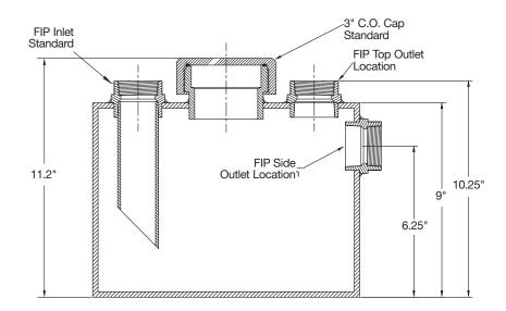
Note: Tanks are made to  $\pm 0.25$  in. tolerance.
