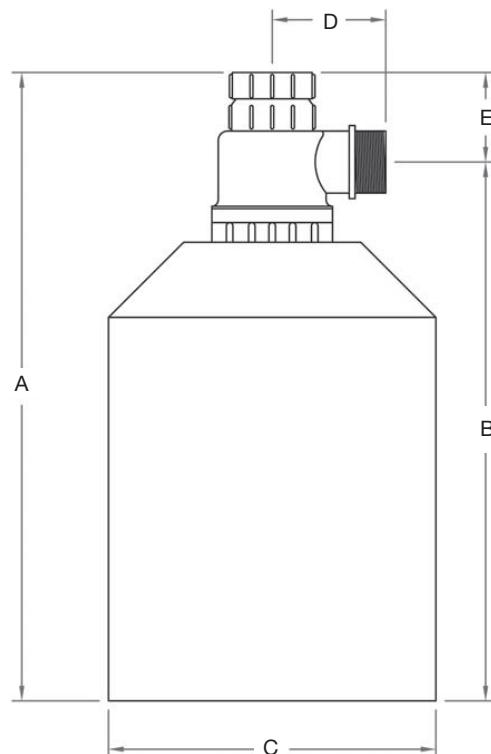
Note: Tanks are made to  $\pm 0.25$  in. tolerance.
