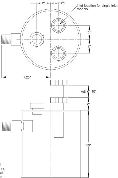
Note: Tanks are made to  $\pm 0.25$  in. tolerance.
