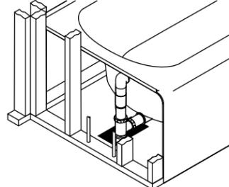
**12** Install the back wall. Insert the back wall tabs into the slots.
