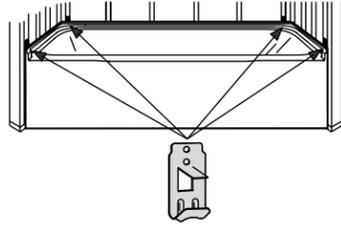
**8** Level the unit. Secure the metal support clips to the studs. Bend the tabs over the flange.
