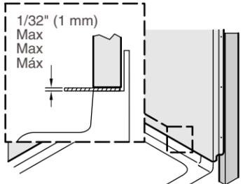
**17** Starting at the bottom, install screws through the dimples to secure the flanges to the studs.
