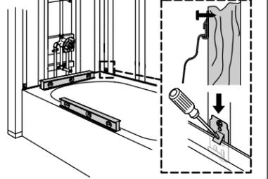
**9** Install plastic attachment clips at all remaining stud locations.
