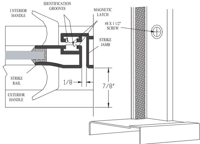
Close the door and check the clearance with the strike jamb. If necessary, loosen the set screws [K] on the top & bottom slide bars and adjust the door panel to align the magnets. When the door panel is properly aligned, tighten the set screws securely.
