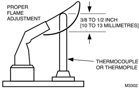
Fig. 8. Thermocouple/thermopile tip must be in pilot flame.
