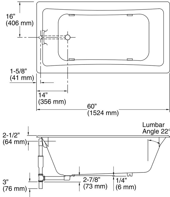
No change in measurements if connected with drain illustrated. (K-7169-AF)
