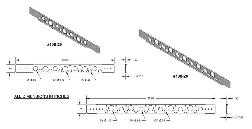
The HOLDRITE® #108-20 and #108-26 are Copper-Bonded™ steel brackets with holes for ½" pipes on 2" centers, holes for ¾" and 1" pipes on 4" centers. Featuring a rolled-edge for added strength, and extruded holes for easier soldering. The #108-20 & #108-26 are designed to positions copper water supplies for urinals, lavatories and other fixtures. When soldering, heat the pipe, not the bracket.
