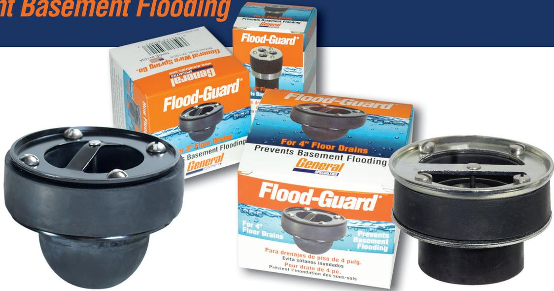
Flood-Guard operates like a check valve to seal off water back-up caused by overloaded sewers. Water flows normally through the drain until the sewer begins to back up. Then the Flood-Guard float rises to seal off the drain opening until the water recedes.
