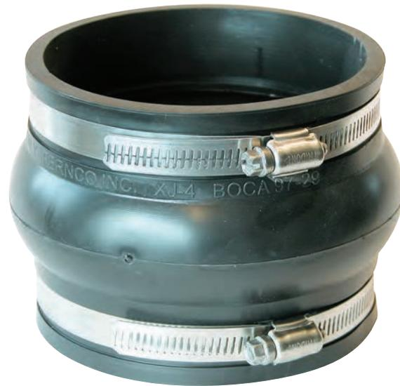
Fernco Expansion Joints will accommodate a maximum of 1-1/2" expansion and 1/2" contraction from a normal position.
