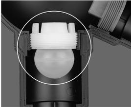
Install as shown into 2" FIP threaded throat of floor drain with ball on the bottom and drainage notches on the top. Be sure to thread completely into drain throat to insure thorough drainage.
