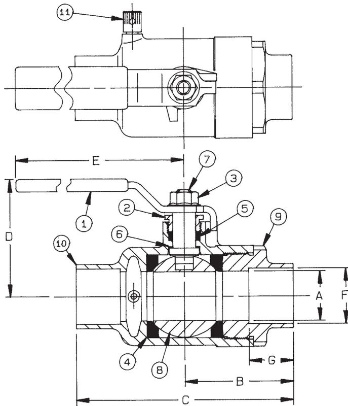
The 95-200 is designed to be soft soldered into lines without disassembly. This allows a tested valve to be installed without disturbing the seats and seals in any way. Soldering temperatures not to exceed 500°F.
