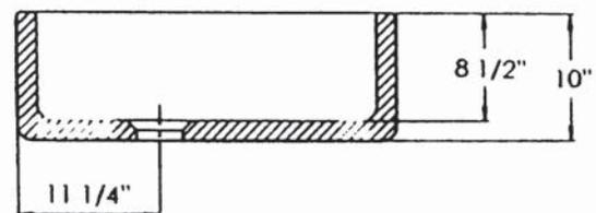
\*NOTE: Due to sink thickness, ISE-type Disposal with Extended Flange #ISE10082 or ROHL 733 Basket Strainer
