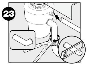
You may need to trim tube for proper fit. Reconnect plumbing (and dishwasher or direct water connection if used). Make sure tailpipe mount is straight.
