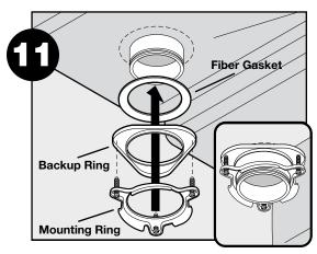
Insert fiber gasket, backup ring and mounting ring. Hold in place while inserting snap ring.
