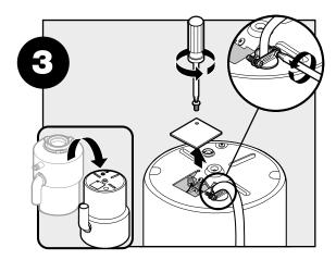
With the electrical supply turned off, flip disposer over and remove electrical cover plate. Save cable connector if applicable.
