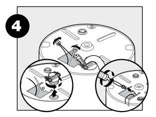
With the electrical supply turned off, disconnect the disposer wires from the electrical supply.
