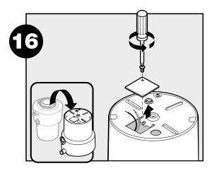
Turn disposer over and remove electrical cover plate. Pull out wires. DO NOT REMOVE CARDBOARD SHIELD.
