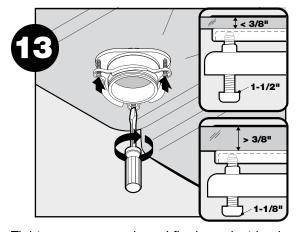
Tighten screws evenly and firmly against backup flange. Use shorter 1-1/8" screws if sink is more than 3/8"thick.
