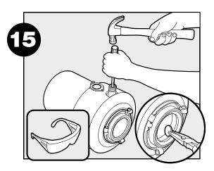
Knock out drain plug and remove plug from inside of disposer.
