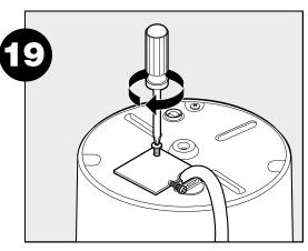
Push wires into disposer (do not displace cardboard shield) and replace electrical cover plate.
