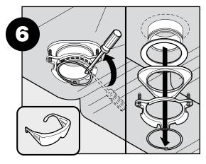
Using a screwdriver, remove the snap ring.
