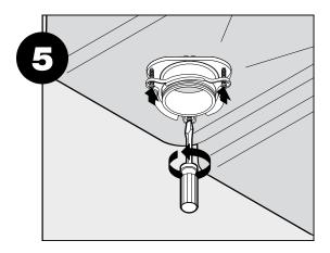
Loosen the 3 screws on the mounting assembly.
