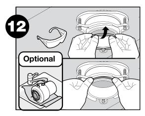
Place a weight such as the disposer on the sink flange to hold it in place. Use a towel to prevent scratching sink. Pull snap ring open and press firmly until it snaps into place.
