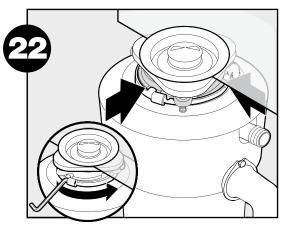
Turn mounting ring until all 3 mounting tabs lock over the ridges on the slide-up ramps.
