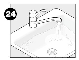
Insert stopper into sink opening. Fill sink with water, then test for leaks.
