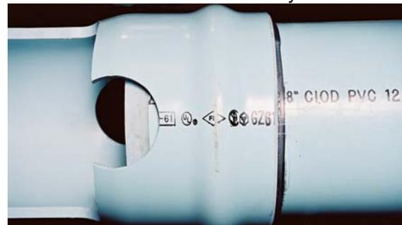
Photo # 11: Properly Inserted Spigot
