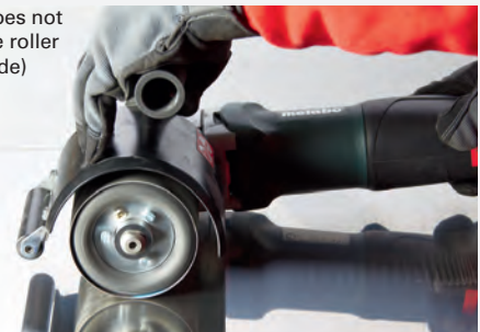
Preparation for mirror polishing: Metabo Burnishers with expansion roller, and Pyramid sanding belts from A160 (120 grit) to A6 (2000 grit).
