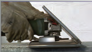
Typical problem...Grinder doesn't reach
