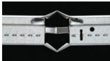
Main beam exposed to fire
