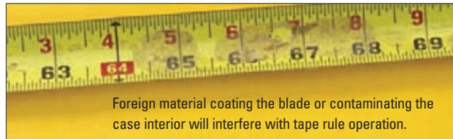
Foreign material coating the blade or contaminating the case interior will interfere with tape rule operation.
