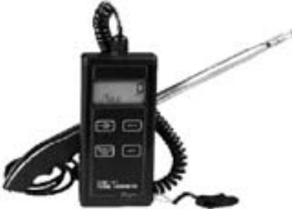
The Series 471 Digital Thermo Anemometers are versatile dual function instruments that quickly and easily measure air velocity in four field selectable ranges, in either feet per minute or meters per second, plus air temperature in °F or °C. High contrast LCD display shows both range selected and present velocity. Convenient backlight provides perfect visibility in low light conditions. Light automatically shuts off after 2-1/2 minutes to prolong battery life. Low battery warning is included.
