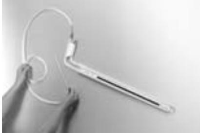
**Above** — Use Series 1227 as a regular U-tube manometer to read high-range pressure on the right leg, or as an inclined manometer (shown here) to read low-range pressure on the bottom leg. Simply incline manometer until fluid levels read zero. No spirit level required. Magnetic clips hold the gage in position on a steel duct surface.
