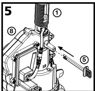
Secure the Motor Assembly/Bottle Support (8) to the Dispenser Assembly (1) shank by pushing the Retaining Clip (5) into place through the vertical slots, until it goes all the way through the Motor Assembly.
