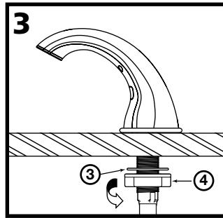
From underneath the counter, first feed the Lock Washer (3) and then the Mounting Nut (4) over the Data Cable (6) and onto the threaded shank of the Dispenser Assembly (1). Be sure that the "teeth" on the Washer will touch the bottom of the counter top and that the Nut threads easily onto the shank. (If the Nut is hard to turn by hand, it is upside down.) Hand-tighten the nut securely.
