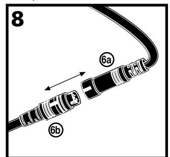
**IMPORTANT:** Connect the two halves of the Data Cable (6a and 6b) by visually lining up the white stripes on each half and gently pushing the cable connectors together until the stripes touch.
