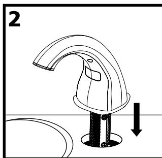
Feed the Data Cable (6) and the shank of the Dispenser Assembly (1) through the hole in the countertop. Point the spout of the Dispenser into the sink bowl and press down firmly on the Dispenser to securely attach it to the countertop.
