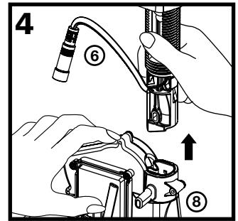
Align the indent inside the top of the Motor Assembly/Bottle Support (8) with the indent on the shank of the Dispenser Assembly (1) and firmly push the Motor Assembly/Bottle Support up, onto the shank.
