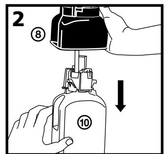
Grasp the empty Refill Bottle **10** with one hand and use the other hand to push the Green release latch on the Motor Assembly/Bottle Support **8** to the right (counterclockwise as seen from above).
