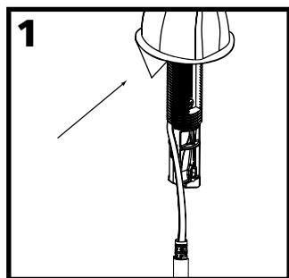
Remove the paper liner from the bottom of the Gasket.
