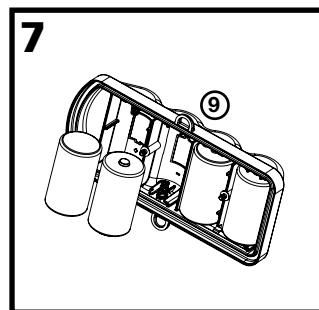
Place four alkaline "D" Cell batteries into the Battery Box (9) cover. The batteries must be positioned according to the diagrams shown on the inside of the cover.
