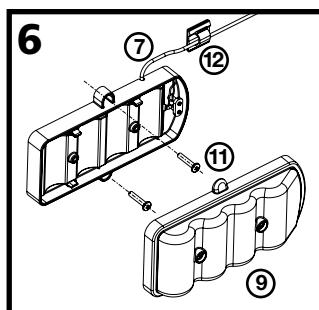
Remove the cover from the Battery Box (9) by loosening the two captive screws on the Battery Box cover. Position the Box on a convenient (vertical or horizontal) surface under the counter top that will allow access for battery changing. Attach the Box to the surface using the two screws (11) and anchors (if attaching to a plaster or masonry surface). Use the Wall Clip (12) to secure the Power Cable (7) to a wall or other under-counter surface if desired.
