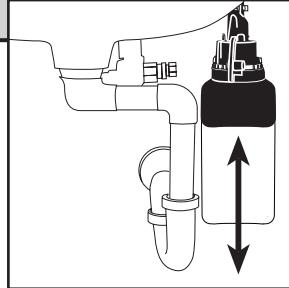
Proper installation allows the unit to vertically hang beneath the sink.
