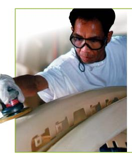
For use on random orbital and rotary sanders. The industry's highest performing film and foam finishing discs are engineered for composite, automotive, and other fine finishing applications. Norton microfinishing film discs produce superior finishes dry without sacrificing cut rate while Norton foam finishing discs are used moist to produce a semi-polished surface to reduce buffing time.
