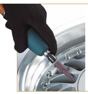
Tapered cone points are strips of abrasive cloth rolled and glued to form a solid shape that is designed to break down during use and reveal the next layer of abrasive. Tapered cone points are similar to cartridge rolls but their shape lends greater accessibility to many difficult-to-reach work areas. They are used for deburring holes and in close tolerance work areas.
