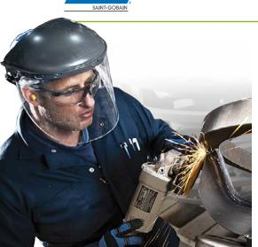
The strongest of coated abrasive discs with resin-over-resin construction on heavy-duty fiber backing. Designed for applications ranging from heavy stock removal to surface blending. Used with back-up pads on portable angle grinders.
