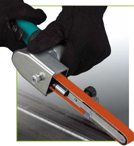
Portable file belt sanders have replaced tedious hand filing and sanding. First introduced in pneumatic, they are now also available in electric. Increasingly, tool manufacturers are introducing additional fixtures for additional applications. The belts listed are popular stock sizes, but additional sizes, specifications, backing materials, and edge scallops are available made-to-order.
