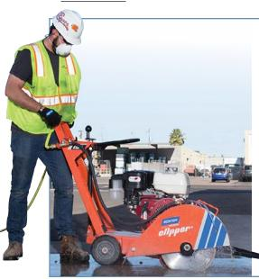
These powerful, self-propelled machines are designed to cut concrete slabs and asphalt and are normally fitted with diamond blades. For inexperienced operators or small jobs, the machines can accommodate these low initial cost, conventional abrasives wheels.
