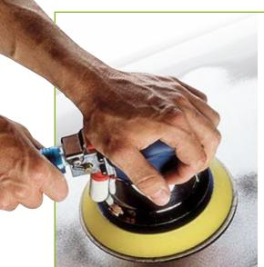
For use on dual action and random orbital sanders. The industry's highest performing and broadest selection of paper discs in PSA (pressure sensitive adhesive) disc rolls and individual discs, and hook and loop discs.
