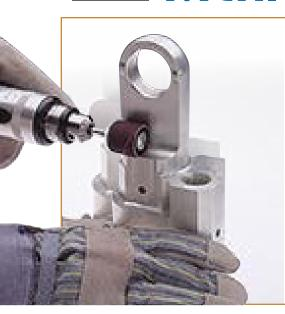
Best product for blending and polishing contours when smooth running is a primary concern. Used for finishing hard-to-reach areas, removing parting lines, imperfections, and burrs on all surfaces.
