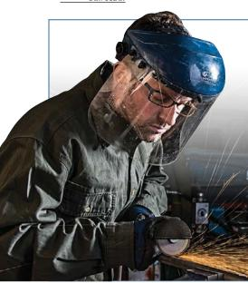
The Norton small diameter cut-off wheel line consists of Type 01/41 straight and Type 27/42 depressed center cut-off wheels from 1-1/2" to 9" diameters. These wheels come in ultra  $\dot{\text{thin}}$  .035" for quick burn-free and burr-free cutting to .125" for more durable applications. All are reinforced for the demanding nature of portable cut-off.
