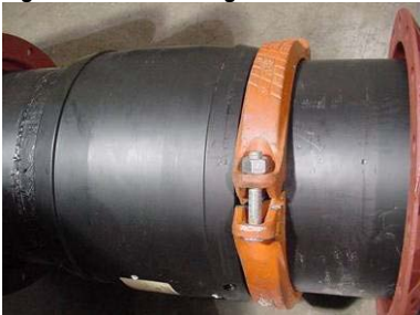
Figure 54: Re-Rounding with Full-Encirclement Ring
