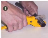
Figure 18 – Installation Instruction for Insert Type Mechanical Coupling
