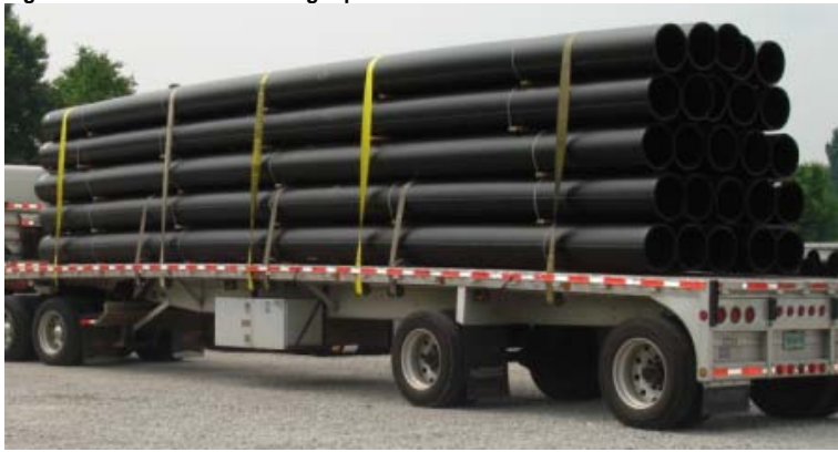
Figure 3: Use Care in Unloading Pipe Bundles
