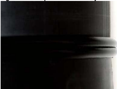
Figure 40: Acceptable butt fusion joint
