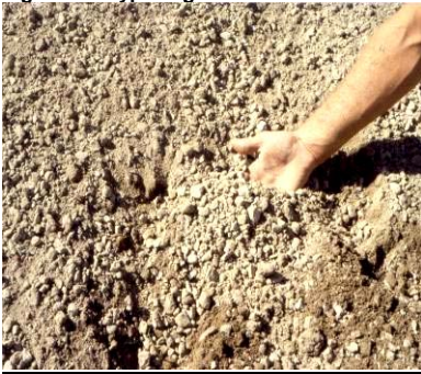
Figure 24: Typical granular embedment
