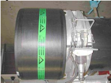
Figure 54: Re-Rounding with Full-Encirclement Ring
