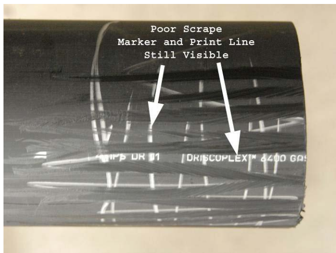
Figure 68: Poor Scrape Unacceptable – Possible Causes: Incorrect Scraper, Poorly Maintained Scraper, Inadequate Number of Passes with Scraper and Ineffective Evaluation of Scraping
