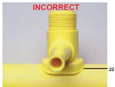
22. Insufficient melt and misaligned
