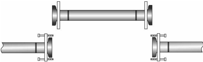
Figure 94: Flange Repair Schematic
