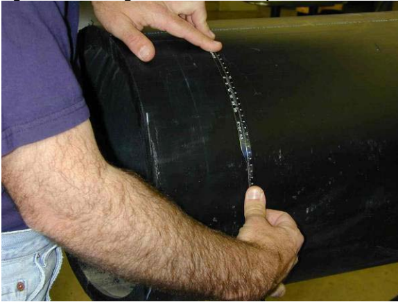
Figure 47: Measuring Diameter with a Pi Tape
