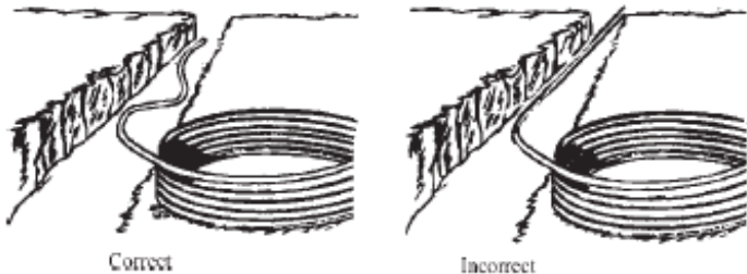
Figure 10: Proper vs. Improper Placement in Trench
