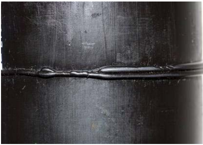
Figure 39: Unacceptable butt fusion joint due to contamination captured in the joint
