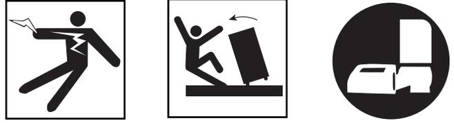
**Set up the Threading Machine and the work area according to these procedures to reduce the risk of injury from electric shock, machine tipping, entanglement, crushing and other causes, and to help prevent threading machine damage.**
