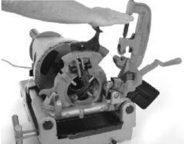
Figure 19 – Closing the Receding Die Head
