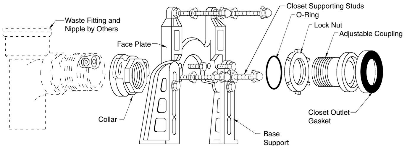
Δ Base support must be securely anchored to floor (with four 1/2" (13) Bolts furnished by others).
