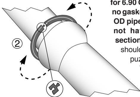
**Step 3** • Assemble the pipe half around the pipe (it may be necessary to insert one bolt with nuts to hold ring segments together). Push the assembled ring and gasket against the face of the pipe bell.
