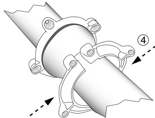
**Step 5** • First, tighten the bolts at the casting joint (where the two halves join). Then, tighten bolt in 20 ft-lbs increments to 40 - 50 ft-lbs.
