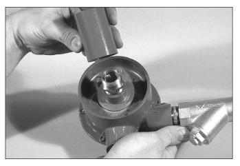
Install the spacer over the jam nut. Make sure the spacer is fully seated over the jam nut.
