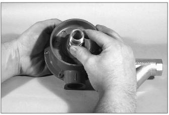
1. Install the jam nut into the alarm motor housing.
