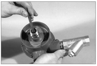
2. Insert the 3½-inch/89-mm long flat drive shaft into the impeller's
