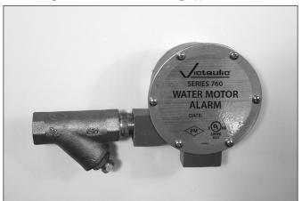
**7a.** Position the housing so that the inlet of the alarm motor housing with strainer is at the 9 o'clock position and the outlet is at the 6 o'clock position, as shown above.
