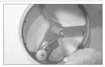
**9.** From the exterior of the building, position the bracket so that the striker will contact the lower portion of the shell.
