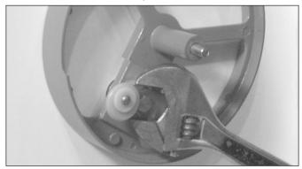
10. While holding the bracket in position, tighten the assembly by using a wrench on the two flats on the striker shaft, as shown above. DO NOT over-tighten the assembly.
