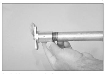
4. Hand-tighten the connecting nipple into the striker assembly.
