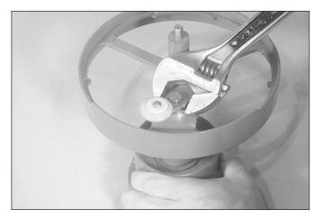
Tighten the assembly by using the two flats on the striker shaft, as shown above. **DO NOT** over-tighten the assembly.
