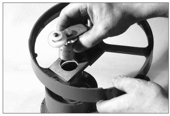
Install the bracket onto the alarm motor housing, along with the striker assembly, as shown above.
