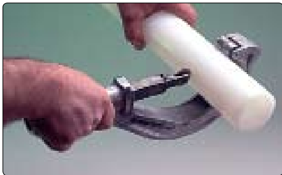
Figure 2: Cut the Tubing
