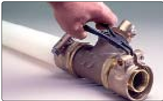
Figure 4: Dismounting Outer Sleeve
