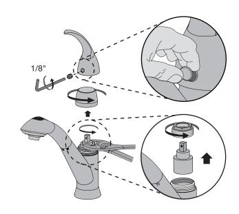
Replacing cartridge and handle
