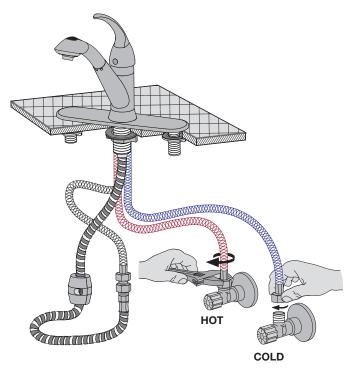
Step 6 Flush supply lines and check for leaks
