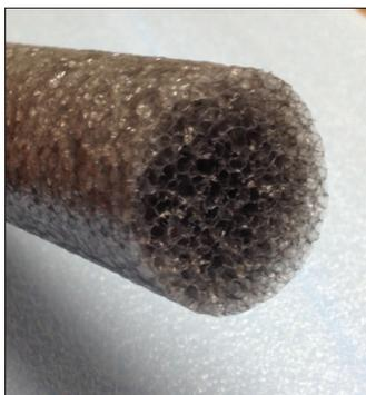
BoMetals Soft Backer Rod (FBRS) is a patented, round flexible polyethylene foam that is used in, but not limited to, expansion & contraction joints, window glazing, curtain wall construction, parking deck, bridge construction, modular home gasketing, & log home chinking.
