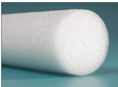
BoMetals Hot Backer Rod (FBRH) is round, flexible continuous lengths of cross-linked polyethylene that is used for backing both hot & cold applied sealants.
