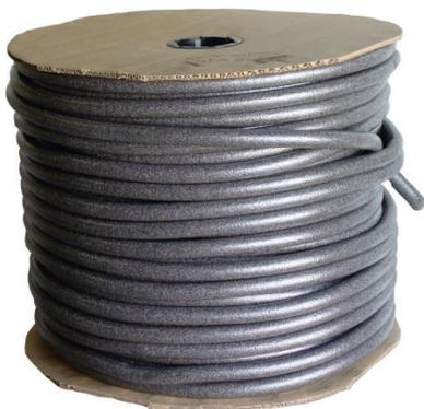
BoMetals Standard Backer Rod (FBR) is a ideal non absorbent compressible polyethylene material inserted into a joint to control sealant depth, creating a backstop to allow proper sealant tooling. It can also be used as a temporary joint seal.
