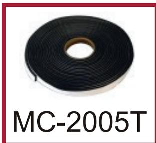
MC-2005T is a 20mm x 5mm (approx. 0.8" x 0.2") chemically modified natural rubber (non-vulcanized) product. The manufacturing process chemically bonds a hydrophilic agent to the rubber. This product is used in concrete joint work where hydrostatic head does not exceed 50 feet. It performs in a wide range of solutions such as seawater or cement water. This material does not contain any toxic substance or heavy metals and is environmentally safe. It comes 320 feet / case.
