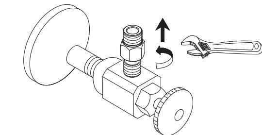
2. Remove the adapter from the water supply by the adjustable wrench.
