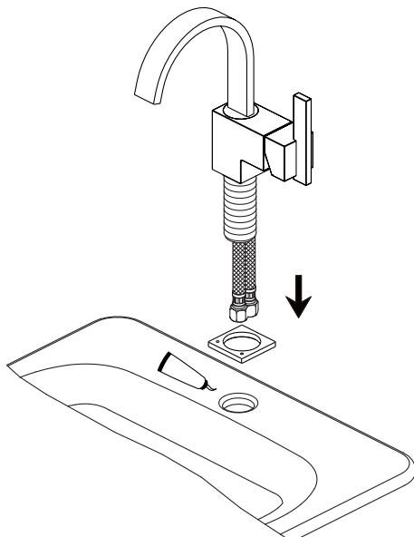
3. From underneath the sink, install the mounting hardware onto the valve shank. Use the phillips screwdriver for final tightening after the body is aligned.
