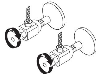
2. Install supply pipes to the valve body.
