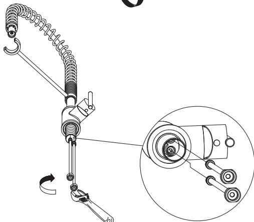
3. Install the faucet body through the top of sink. If your sink has three holes in the deck, refer to drawing B, install the faucet using the deck plate DA665051 (Sold Separately).
