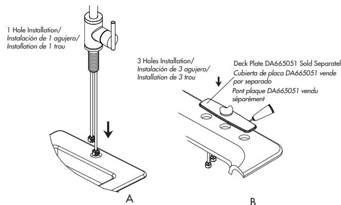
4. From underneath the sink, install the mounting hardware onto the valve shank. Use the phillips screwdriver for final tightening after the body is aligned.
