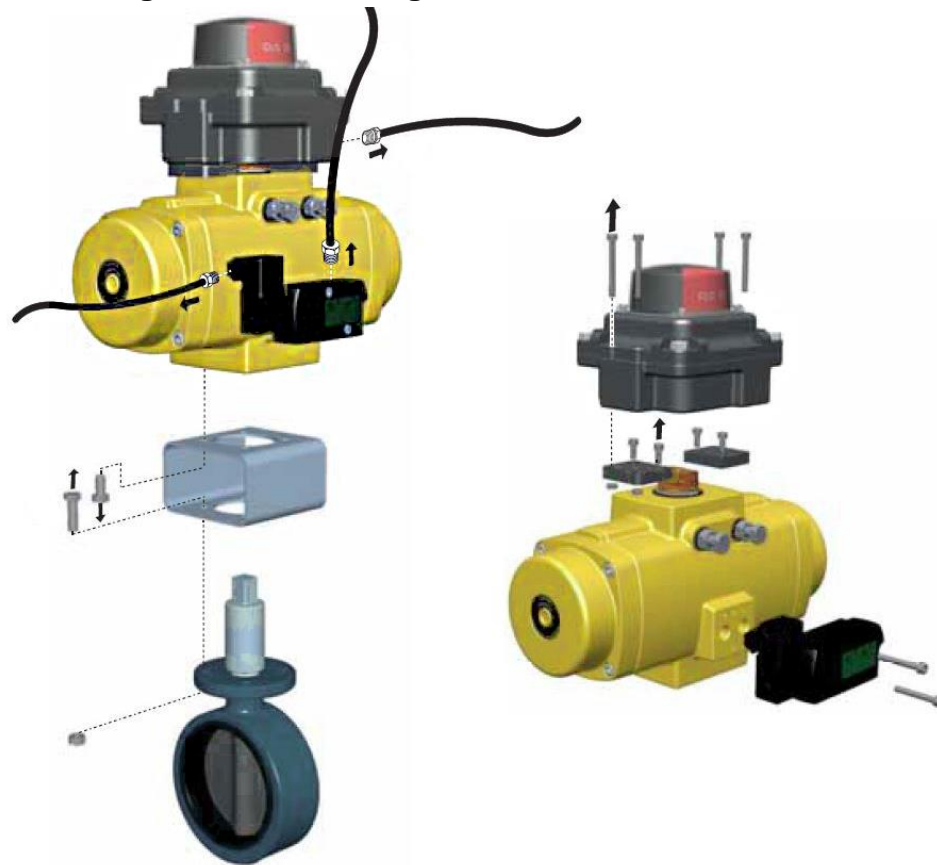
Figure 14: Removing Actuator from Valve/Bracket
