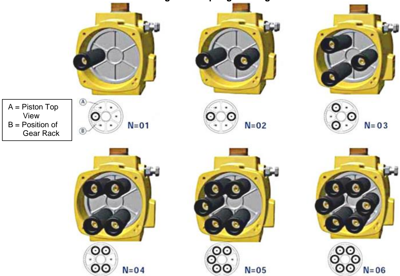
Figure 27: Spring Cartridge Placement
