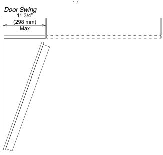
**NOTE**: Additional space needed depending on the thickness of front panels and handle used.
