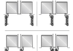
If there is a partition with a thickness from  ${}^5/{}_8$ " (16 mm) to 6  ${}^5/{}_{16}$ " (160 mm) between the adjacent appliances, then each appliance should be individually installed within its own niche using the mounting accessories included. The "Merging Kit" will also be needed.
