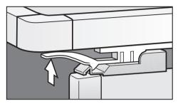
■ On both sides of the container, pull the latches (see arrow) upward and lift the container out of the freezer
