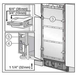
The installation aids ③ on the appliance door have been designed for custom door thicknesses of 3/4" (19 mm) and 1 1/2" (38 mm).
