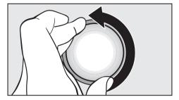
■ Turn the light cover counterclockwise and pull out.
