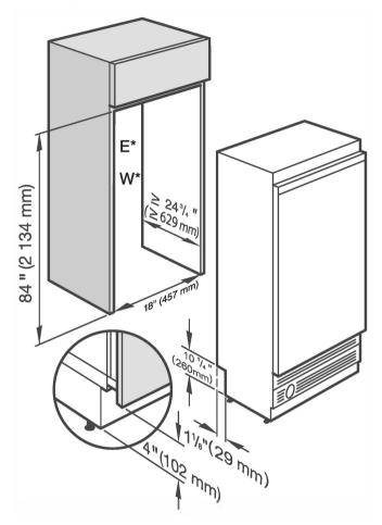
E\*: The position of the electrical connection should not be higher than 9" from the floor.
