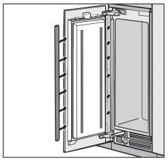
■ To mount the cover strips on both sides of the door, click them into place from bottom to top, into the gap between the appliance door and the custom door.
