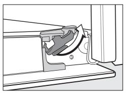
Release the locking clamps by turning them as far as they will go. Do not attempt to take the door off the brackets when it is in the horizontal position, the brackets will spring back against the oven.
