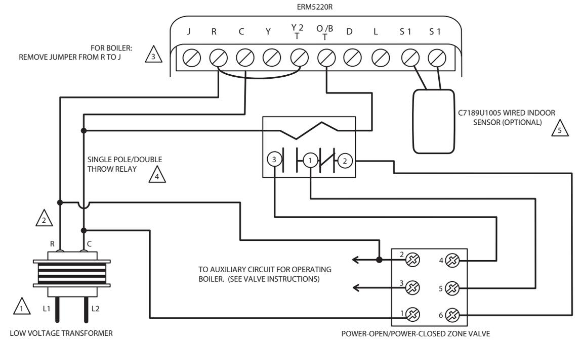
WIRING AT THERMOSTAT IF CUSTOMER ALSO HAS FORCED AIR COOLING
