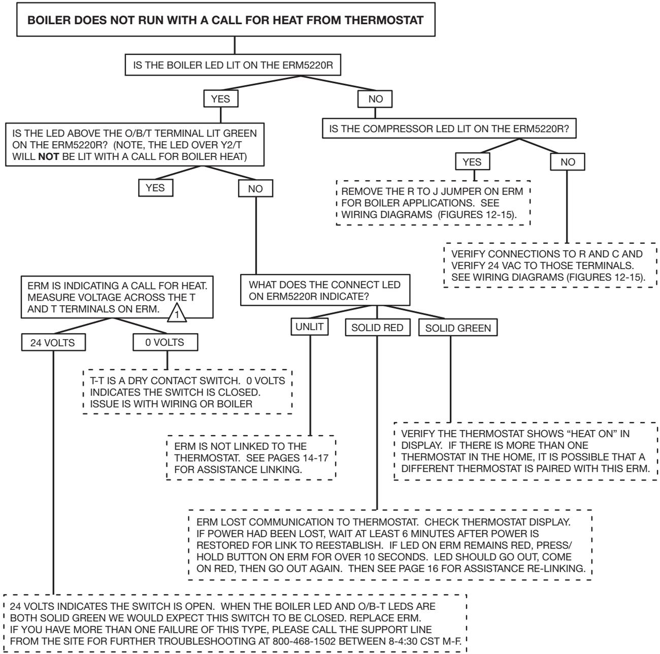
**1** YOU CANNOT TEST THESE TERMINALS WITH A CONTINUITY METER. WHEN WIRES ARE NOT CONNECTED TO THESE TERMINALS, THERE WILL BE INFINITE RESISTANCE ACROSS THE TERMINALS WHETHER THE DRY CONTACT SWITCH IN THE ERM IS OPEN OR CLOSED. ONLY TEST WITH THE WIRES CONNECTED.
