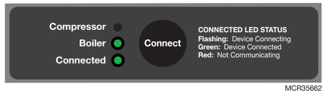
15. Back at thermostat, display will indicate that the Equipment Remote Module has been added. Press “Done”.
