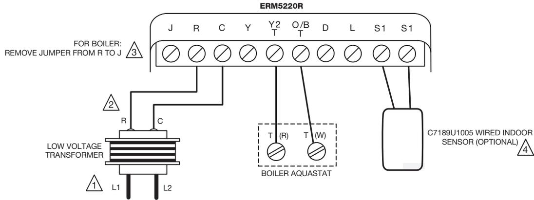
WIRING AT THERMOSTAT IF CUSTOMER ALSO HAS FORCED AIR COOLING OR A HYDRO-AIR APPLICATION (NOT REQUIRED ON HEAT ONLY APPLICATIONS)
