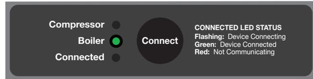
3. When the thermostat is powered it will prompt you to select whether the system is residential or commercial. After setting residential or commercial and choosing the thermostat name, the display shows the below screen (setup 110).
