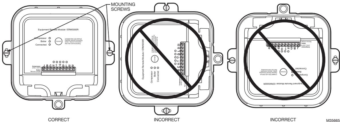
**Fig. 6. Mounting orientation.**
