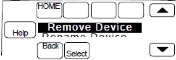
11. Scroll down until “Equip Rem. Module” is selected. And press “Select”. Display says “Remove Equip. Rem. Module?” Select “Yes”.
