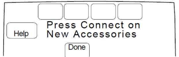
14. Press/release the “Connect” button on the ERM5220R. After releasing the button, the connected” LED should flash green and then turn solid green.
