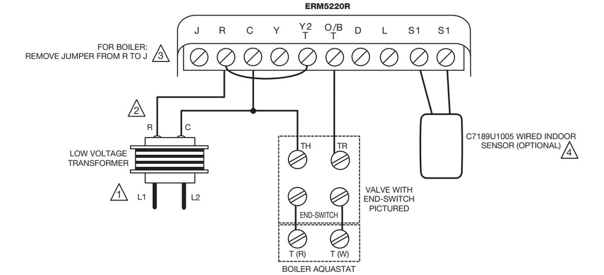
WIRING AT THERMOSTAT IF CUSTOMER ALSO HAS FORCED AIR COOLING OR A HYDRO-AIR APPLICATION (NOT REQUIRED ON HEAT ONLY APPLICATIONS)
