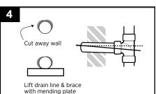
Adjust drain to achieve pitch only if standing water is present (code requires 1/4" drop per foot of drain line for proper pitch). Seal wall according to code.
