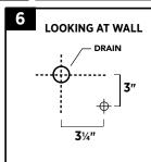
Install 1/2" x 3/8" compression straight stop with the handle facing floor.
