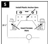
Measure and mark rough in. If in-wall carrier is not used. Use a 5/16" masonry bit to drill hole, then install the hanger bracket with one plastic anchor and screw.
