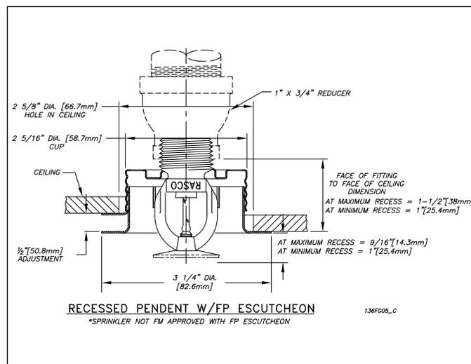
**Note:** A leak tight 1/2" NPT (R1/2) sprinkler joint can be obtained with a torque of 8 - 18 ft-lbs (11 - 24 N-m). Do not tighten sprinklers over maximum recommended torque. It may cause leakage or impairment of the sprinklers.
